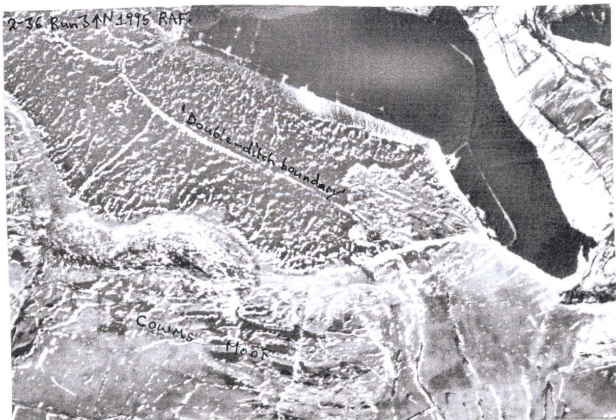
Fig. 6.8. A section of a recent aerial photograph, taken after a light fall of snow, which highlights the fan-shaped peat cutting on Hey Ridge, Alport Dale. The gathered snow defines the peat cutting face, some of the service tracks on the overcut area, and the associated drains/boundary features. The dark, sub-rectangular patches, towards the bottom of the photograph, define remnants of topogenous mire on Cowms Moor.
