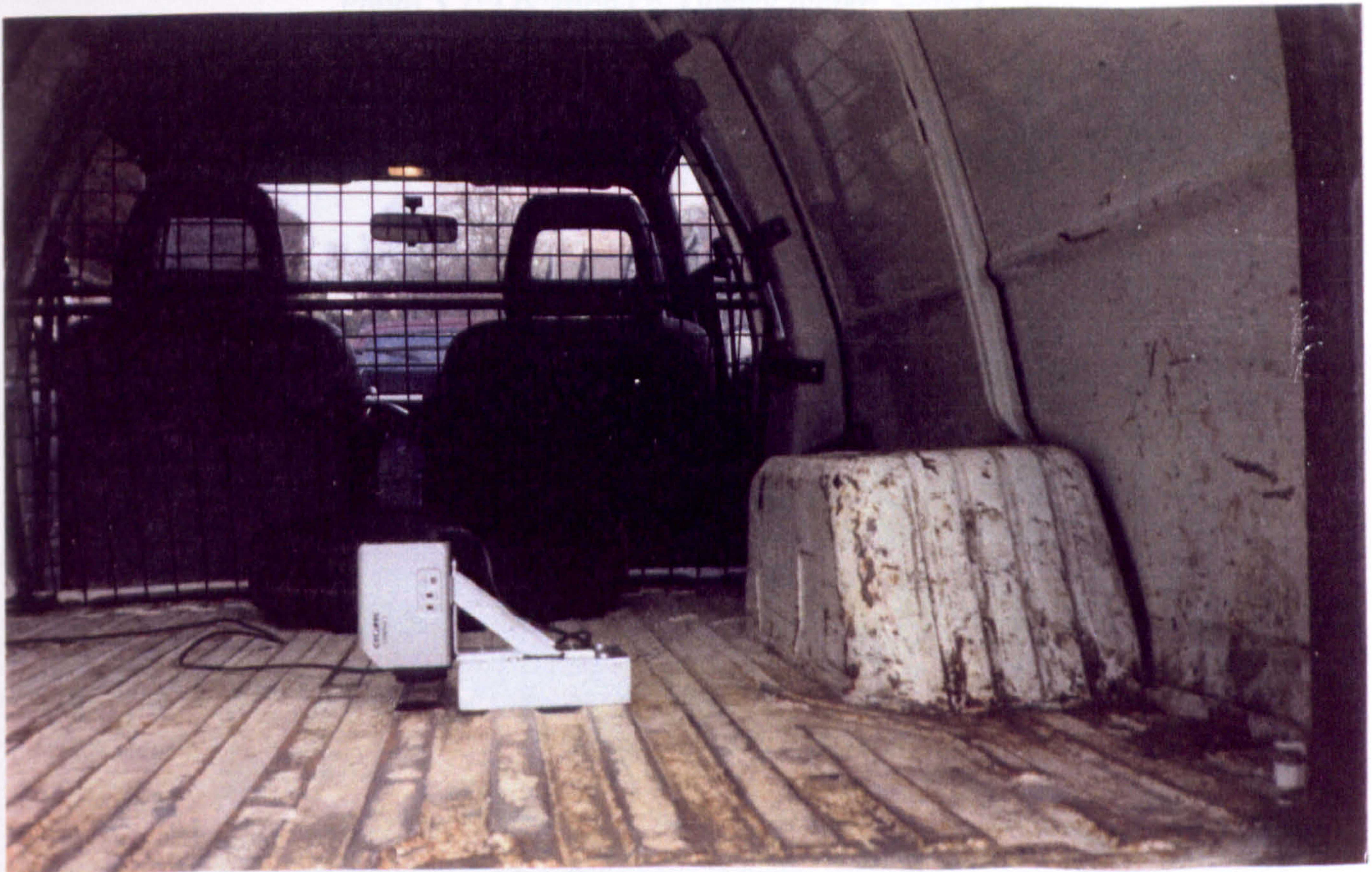
Photo 3.5: IRT On Mounting In Back Of Van
