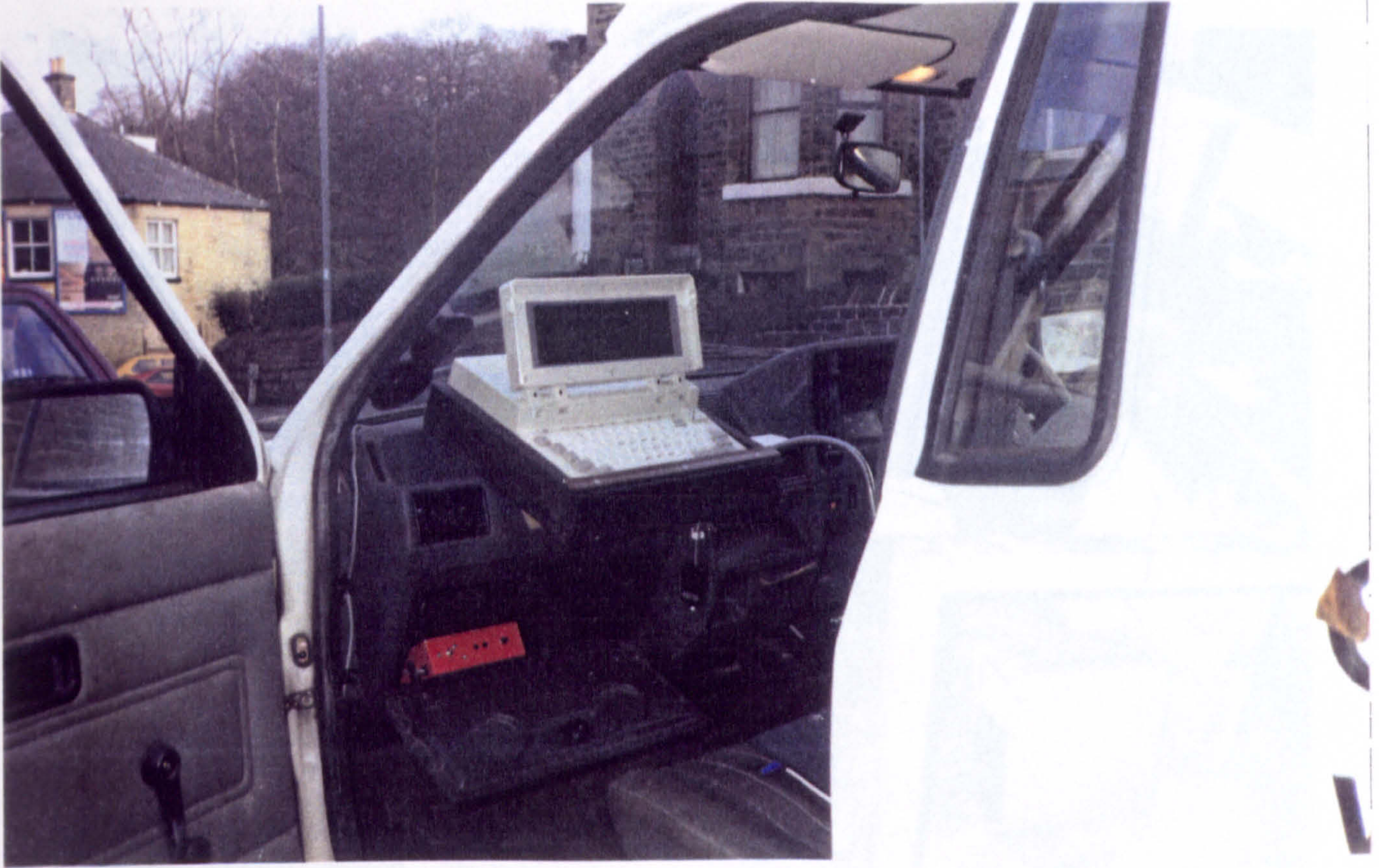
Photo 3.4: Electronics Box And Computer Mounting In Van
