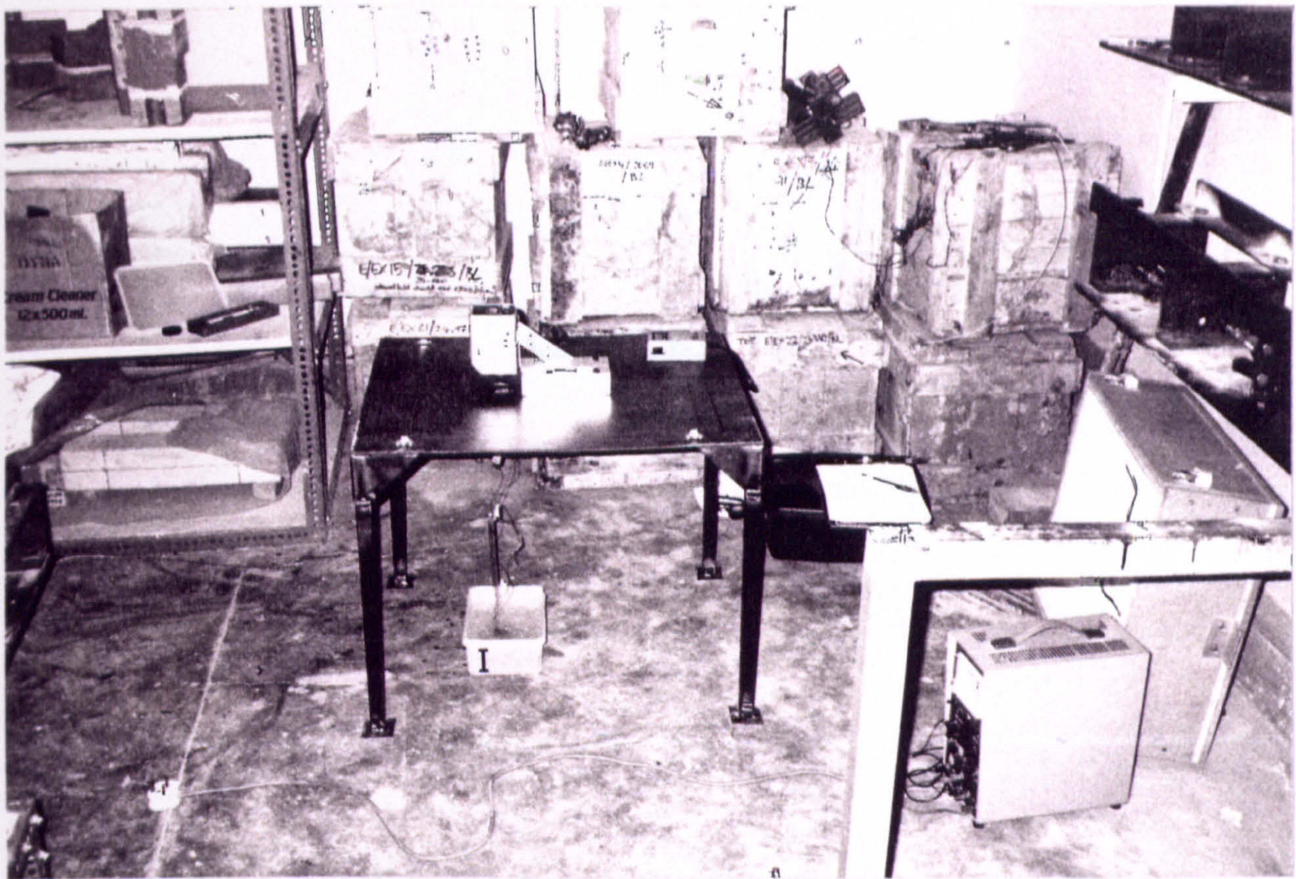
Photo 3.6: Testing Performance Of IRT Using Melting Ice (I) As Target
