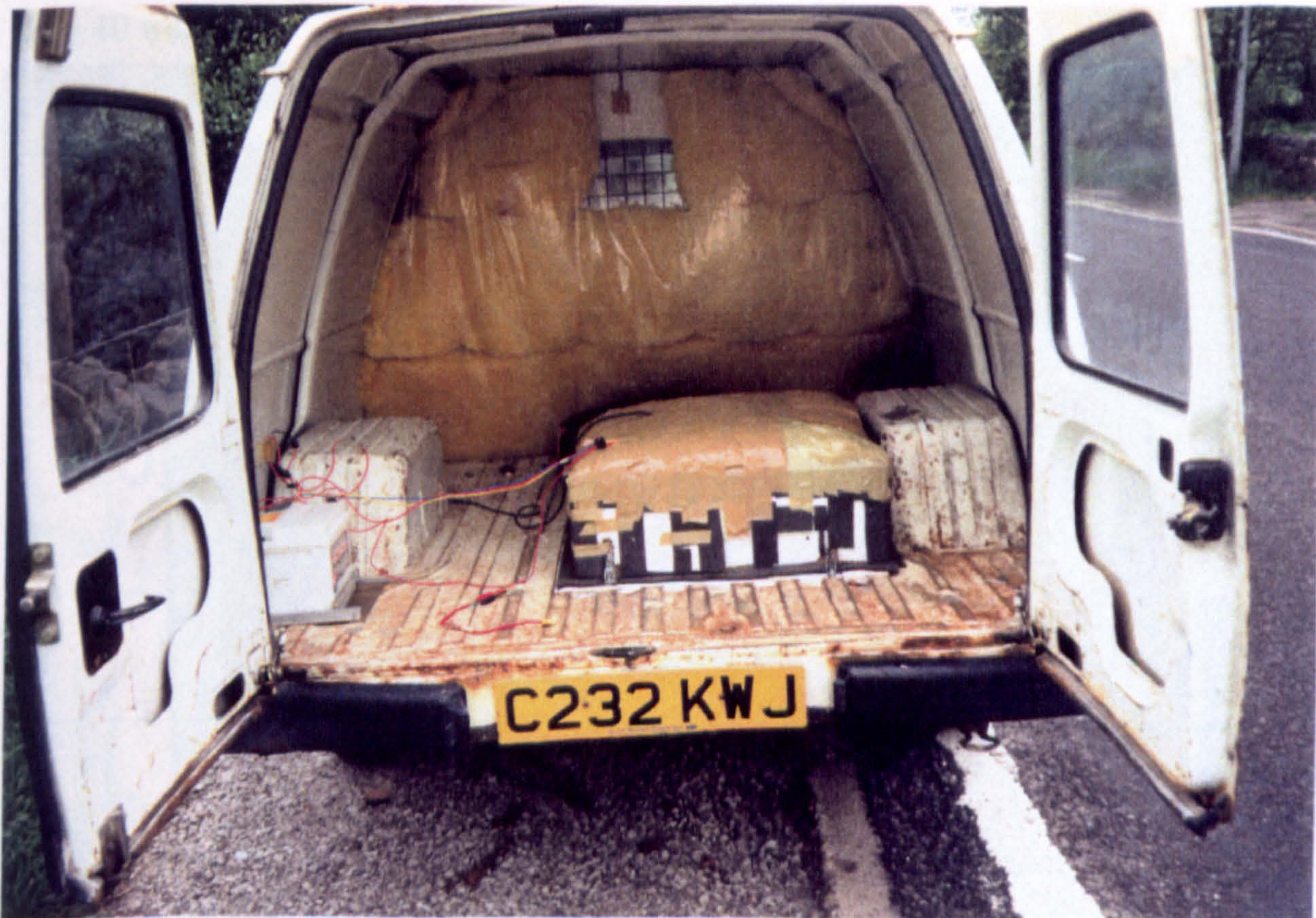
Photo 4.6: Temperature Control Box Used in Van 1989/90 With Insulation
