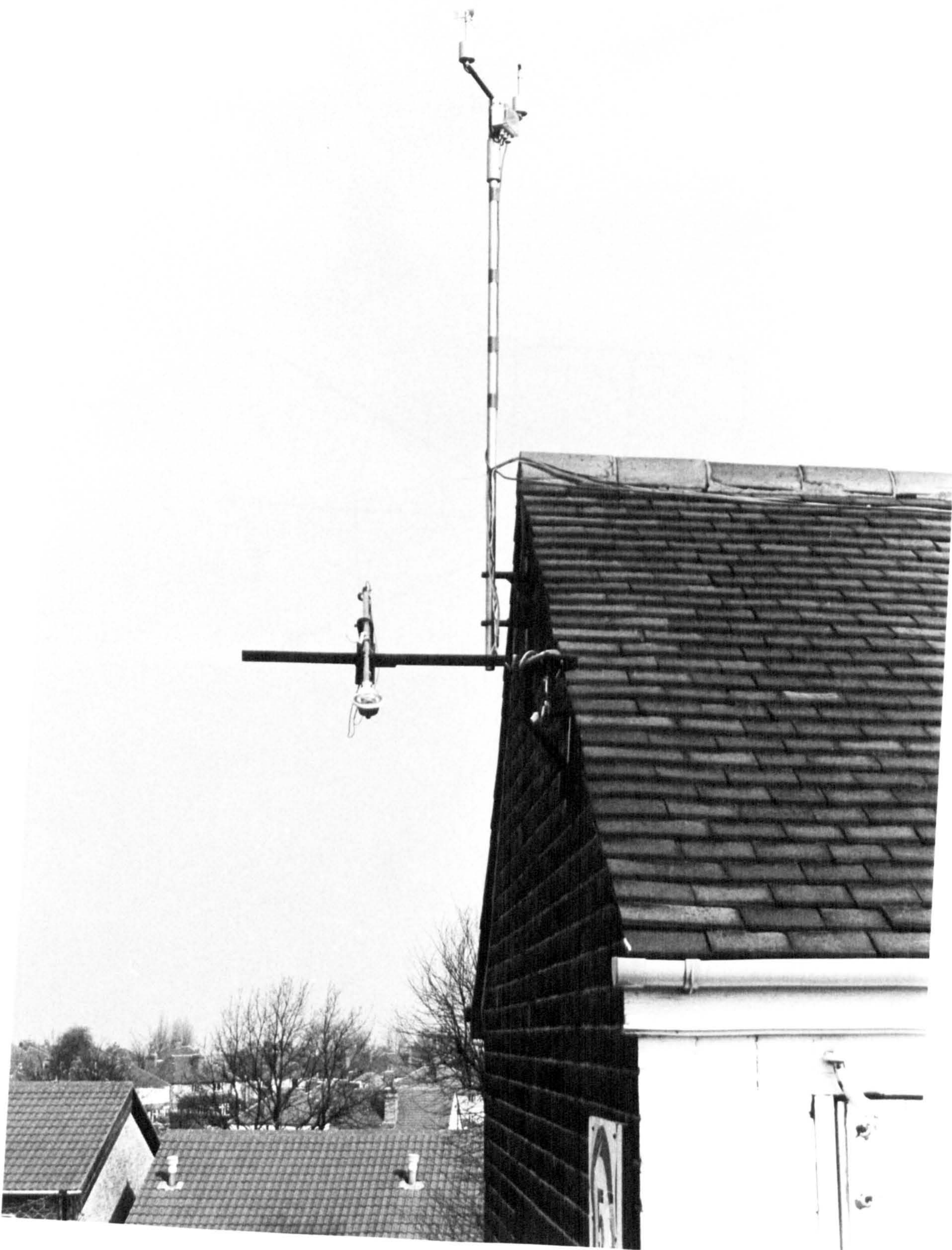
Figure 4.11 Gable end mounted anemometer, wind vane and net radiometer
