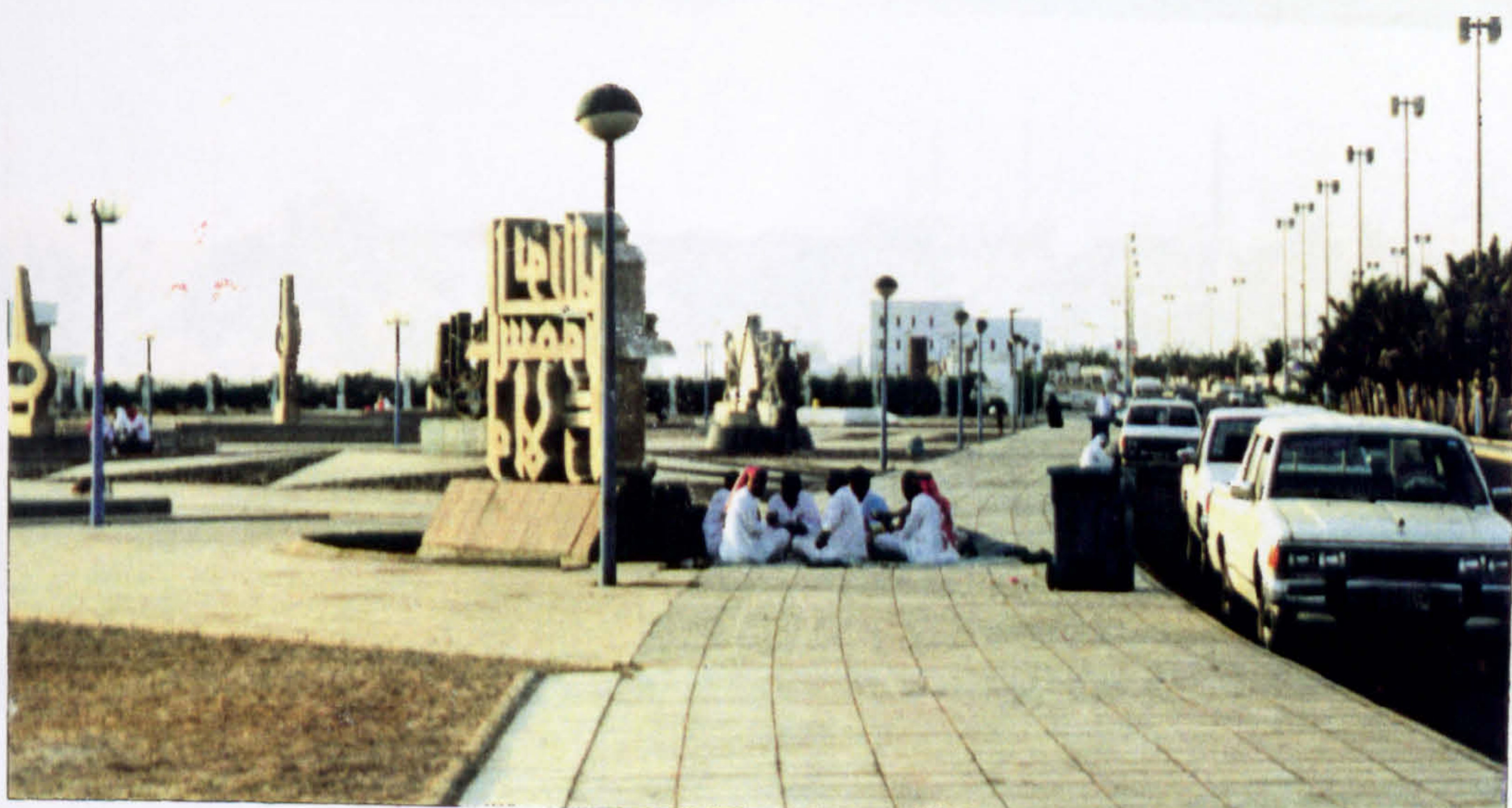
FIGURE 6.18 A typical pavement design of recreational provision where the overall design of pavements or side walks were not planted to be for continuous pedestrian movements, with easy accesses for handicapped people. It is very difficult, if not impossible, to wheel chair people to move along side pavements.
