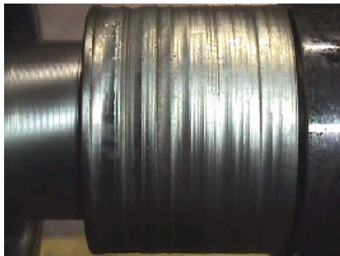
Figure 35 Erosive wear of a pump casing[36]
