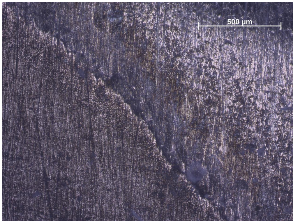
Figure 82 Surface treatment failure (surface remaining on bottom left side of image)
