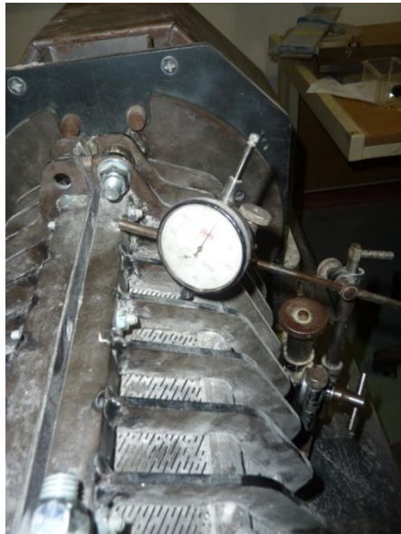
Figure 137 Dial gauge positioning
