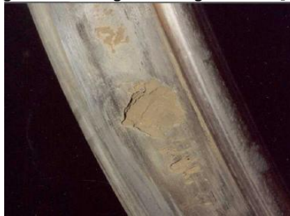
Figure 26 Surface fatigue of rail wheel[26]
