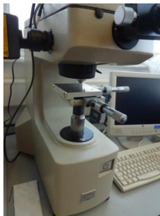
Figure 65 Micro hardness indent test set up
