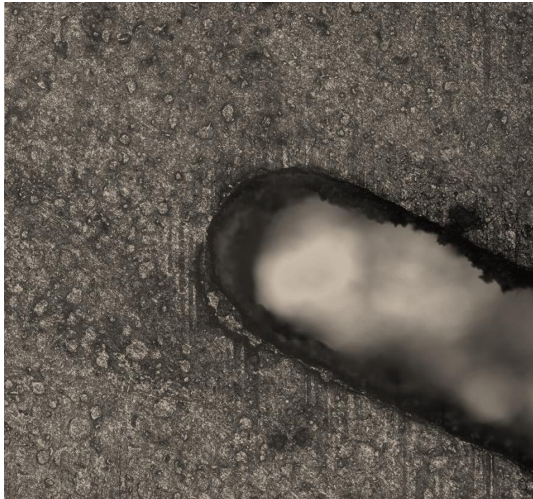
Figure 76 Microscope image of unworn screen slot
