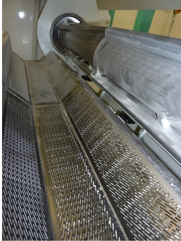
Figure 23 Perforated Screens in Replacement Position
