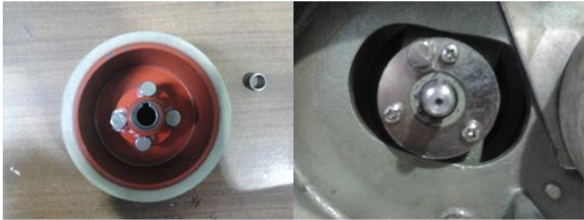
Figure 113 Magnet layout on roller (left) and casing (right)
