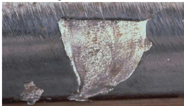
Figure 34 Delamination of a gear tooth[32]
