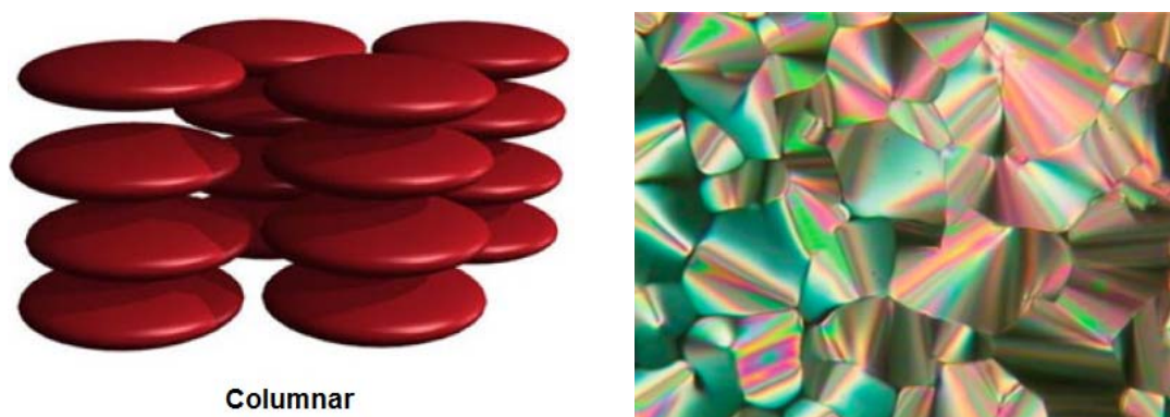
Figure 1.13 Columnar phase and its texture (reproduced from I. Dierking, Textures of Liquid Crystals , WILEY-VCH Verlag GmbH & Co. KGaA, Weinheim, 2003)
