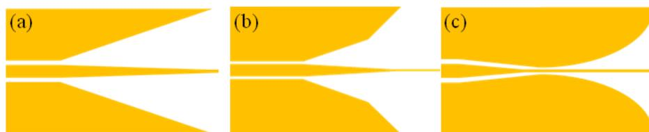
Figure 1.14: Different geometries of CPW – PGL transitions defined with (a) single stage linear transition [91], (b) a double stage linear transition [92] and (c) the curved transition of the ground planes [91].
