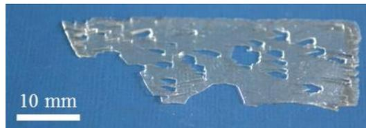
Figure 3.31: Photograph of the quartz after substrate thinning using HF wet etching.
