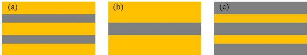
Figure 1.10: Aerial view of (a) CPW, (b) CPSlot and (c) CPS. Yellow represents the metallization and the grey represents the substrate material.
