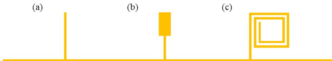
Figure 5.2: Stub filters using (a) quarter wavelength stub, (b) dual impedance quarter wavelength stub and (c) spiral rejecters.
