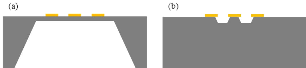
Figure 1.12: (a) A simplified schematic of a CPW on a membrane substrate as demonstrated by references [74, 80, 81]. The waveguide (yellow) is defined on the membrane using standard cleanroom processing before the material beneath the waveguide is etched away using wet etching. (b) A simplified schematic of a coplanar-air transmission lines demonstrated by references [84, 85]. The waveguide is defined similarly to (a) except the material is etched top down from between the metal.
