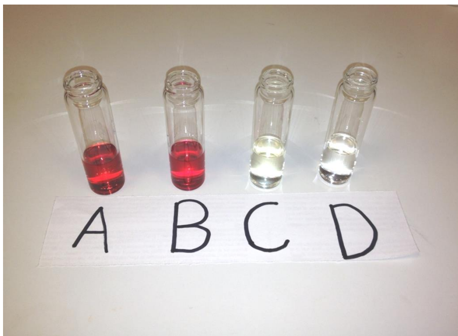
Figure 3-1. Image of dried H. sabdariffa extracts extracted by using different solvents, (A) water extract, (B) methanol extract, (C) ethyl acetate extract (D) hexane extract
