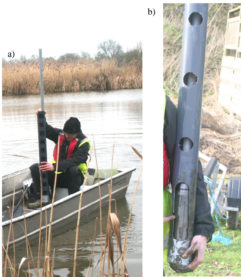
Figure 2-10: a) bringing the corer to the shore, upright with sample inside the inner tube b). detail of the inner tube with undisturbed sample inside. Holes were drilled on the outer pipe to allow water to drain easily when retrieving the corer and to have a better grip when pulling the tubes against the suction of the sediments
