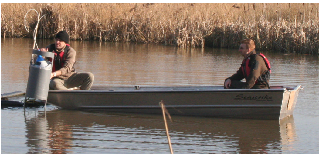
Figure 2-6: Deployment of a benthic chamber. Sections of the pipe that would not be part of the benthic chamber were removed, to make the chamber lighter and to minimise the suction effect when the chambers needed to be pulled out of the sediment.
