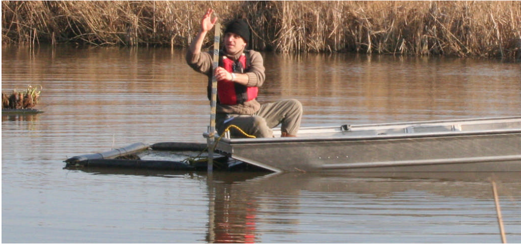
Figure 2-2: Dipping the pond using a flat bottomed graduated wooden staff in October 2010. The boat is secured to one of the unvegetated rafts. On the left of the photograph, another raft can be seen with some vegetation on it
