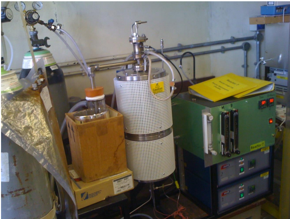
Figure 3-3 Photograph of the ultra-high temperature up-draft reactor
