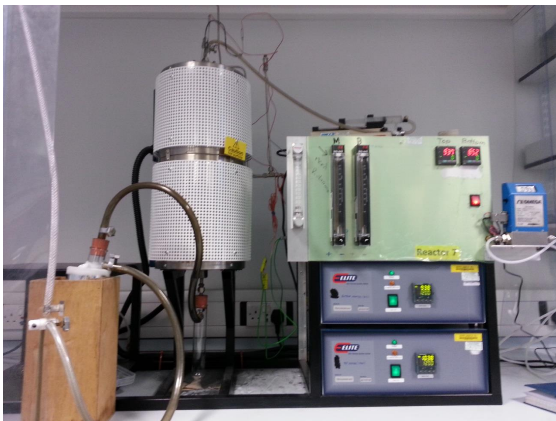
Figure 3-6 Photograph of the ultra-high temperature down-draft reactor
