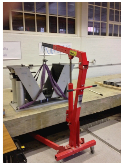
Figure 6-1- placing the TMD on the slab
