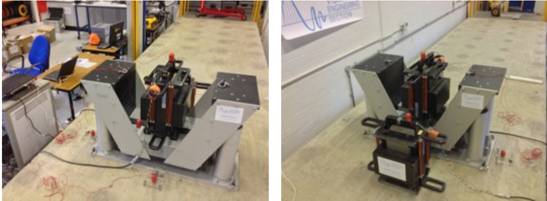
Figure 6-14- HTMD and instrumentation arrangements on the laboratory structure (back and front view)
