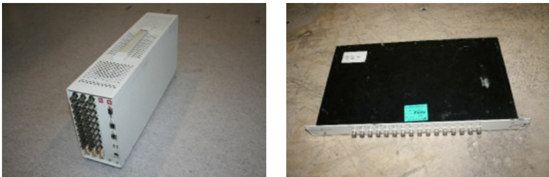
Figure 6-4- Spectrum analyser (left) and signal conditioner (right)
