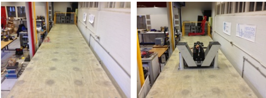
Figure 6-12- Laboratory slab strip; empty (left) and attached with HTMD (right)
