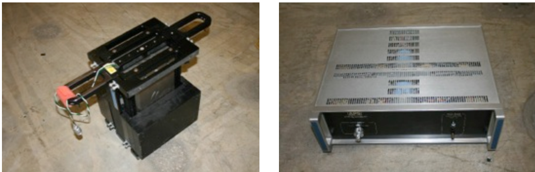
Figure 6-3- Shaker (left) and amplifier (right)
