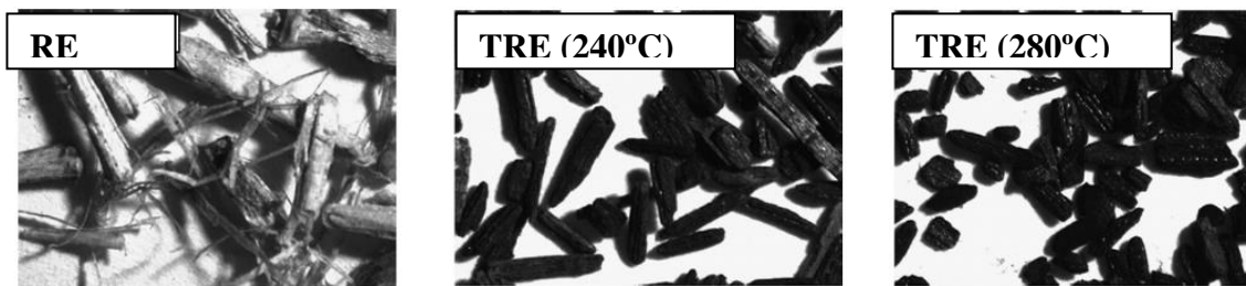
Figure 3.9. Images of raw eucalyptus (RE), torrefied eucalyptus (TRE) at 240°C and 280°C respectively (Arias et al. , 2008).
