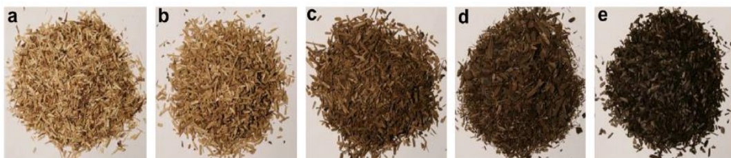
Figure 3.8. Images of willow: a) untreated; b) low temperature, short residence time; c) low temperature, long residence time; d) high temperature; short residence time; e) high temperature, long residence time (Bridgeman et al. , 2010).
