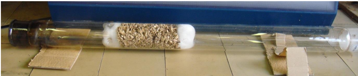
Figure 4.3. How biomass fuels are positioned inside the reactor tube. The biomass shown in the above picture is eucalyptus.
