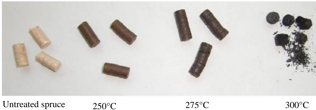
Figure 8.10. Pellets of spruce and torrefied spruce of increasing temperatures (250, 275 and 300°C) (Stelte et al. , 2011).
