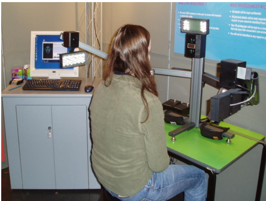
Figure 2.3 - Geometrix® FaceVision802 3D digital stereographic scanner.
