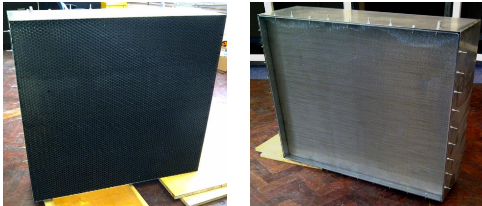
Figure 4.8 Design of the honeycomb screen flow straightener for the closed-loop wind tunnel
