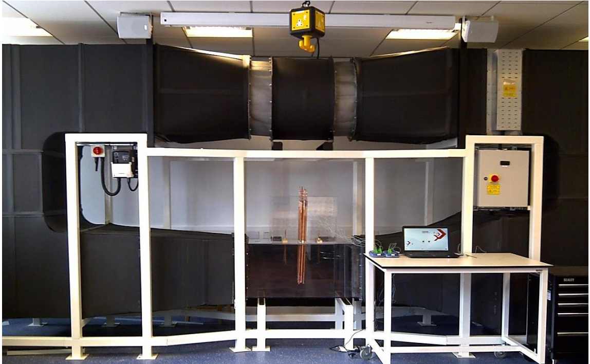
Figure 4.1 University of Leeds closed-loop wind tunnel side elevation
