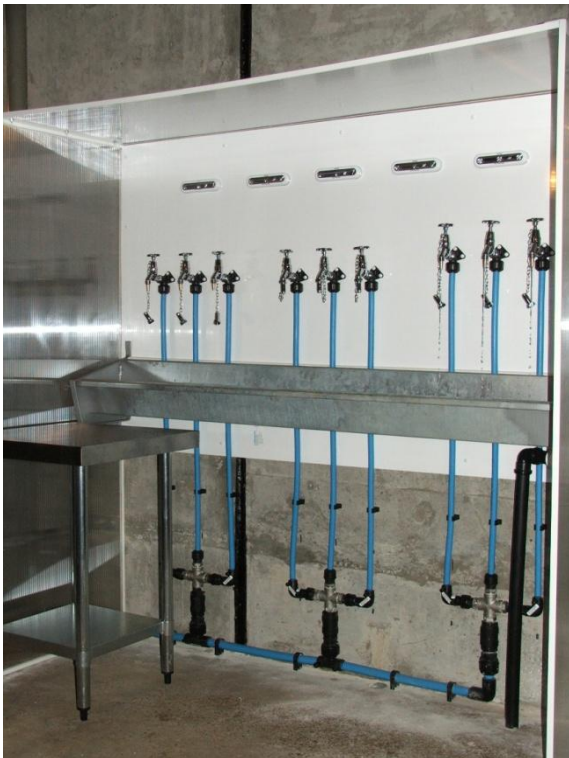
Figure 42: Tap rig designed and commissioned to investigate methods of protecting sample taps from environmental contamination.
