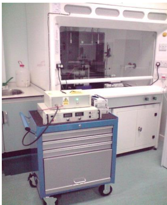
Figure 4.2. Picture of the electrospinning system used in the project, within a chemical hood at the School of Clinical Dentistry of The University of Sheffield.
