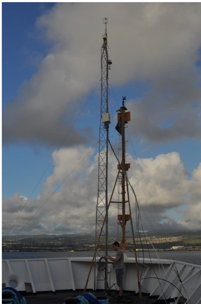
Figure 5.11 – Air sampling inlet secured at top of bow tower 10 m above sea level and adjacent to sonic wind measurement for flux calculation.
