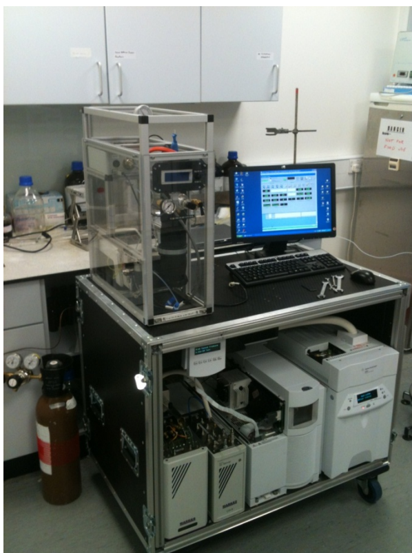
Figure 2.17 – Field portable TD-GC-MS system mounted in flight case. AutoP&T system (section 2.6.2) mounted on top.
