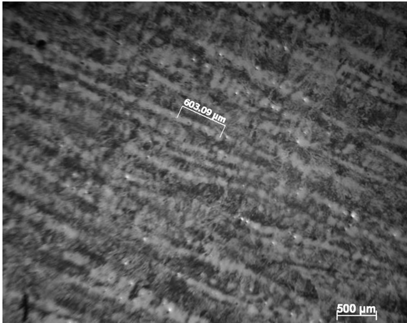
Figure 5-6: Secondary dendrite arm spacing measurement at 23 mm depth.
