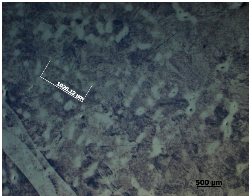
Figure 5-14: Secondary dendrite arm spacing measurement at 115 mm depth.
