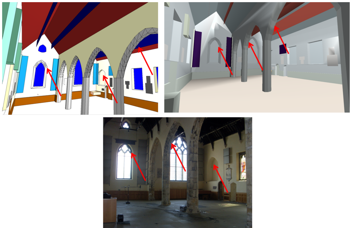
Figure 5.19 Modelling arches between the columns and at the top of the windows using subdivision of surfaces. On the top left, the CATT-Acoustic model is represented, on the top right, the ODEON model, and at the bottom, the actual space is pictured.
