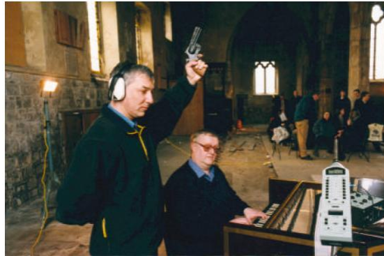
Figure 5.24 Evidence for the gunshot method used by Arup Acoustics for the acoustic measurements carried out in St. Margaret's Church during the development of the space in 1998 [185].
