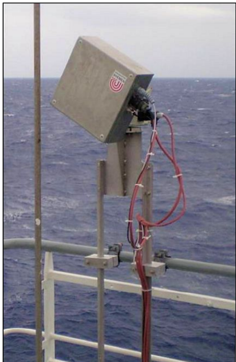
Figure 5.9. The University of Bremen MAX-DOAS telescope installed on the starboard side of the upper deck of the RV Sonne . The red Y-shaped optical fibre bundles leave the telescope and transmit light to the two spectrometers, housed in an indoor laboratory. Photograph by Dr Folkard Wittrock, University of Bremen.
