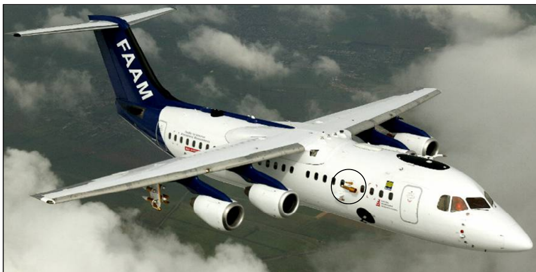
Figure 2.2. The BAe-146 G-LUXE research aircraft in flight, showing the FAGE Eisele inlet (circled) on the starboard side of the aircraft (see section 2.4.3). Photograph by David McIntosh of BAE Systems.
