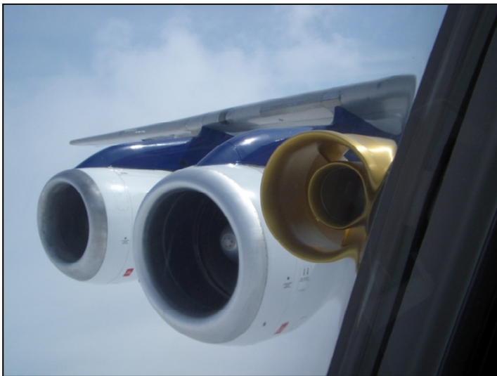
Figure 2.6. Photograph of the FAGE Eisele inlet from inside the aircraft, showing concentric cylinders. Photograph by Dr Jim McQuaid.
