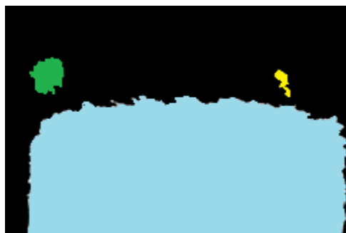
Figure 7-7: Object segmentation example: each object was attributed a different colour on the image
