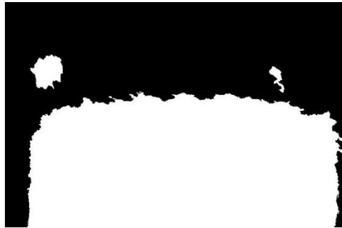
Figure 7-5: Binary image obtained from Figure 7-4 after thresholding (white - tablet and particles, black - background)
