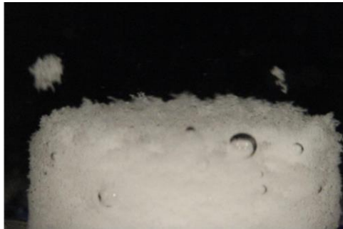
Figure 7-4: Typical colour image generated using the flow cell during tablet dissolution in water
