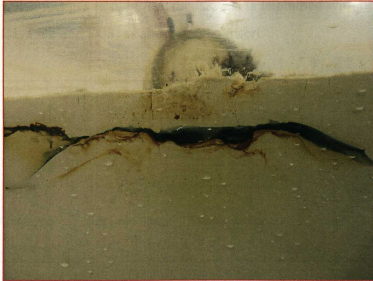
Figure 4- 8: Side view of tank showing chemical alterations of the soil sample
