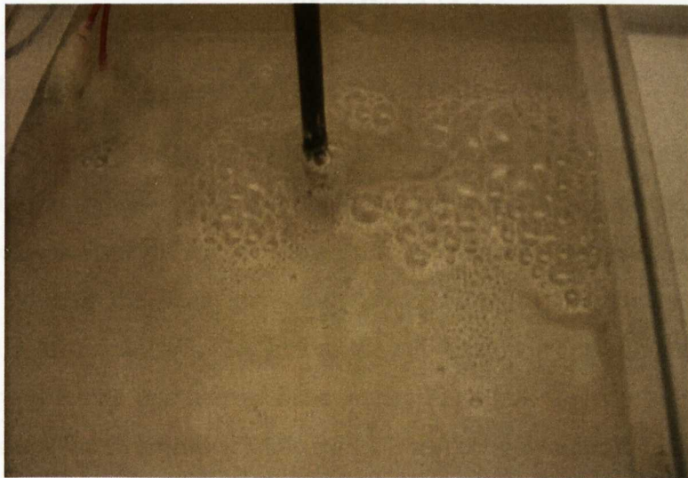
Figure 4- 26: Gas escape from the soil during EK treatment
