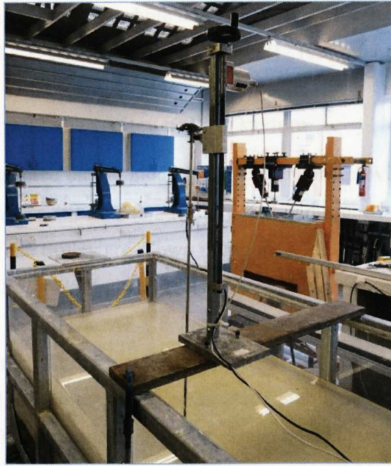
Figure 3 - 20: Set up for T-bar penetrometer testing in the big tank
