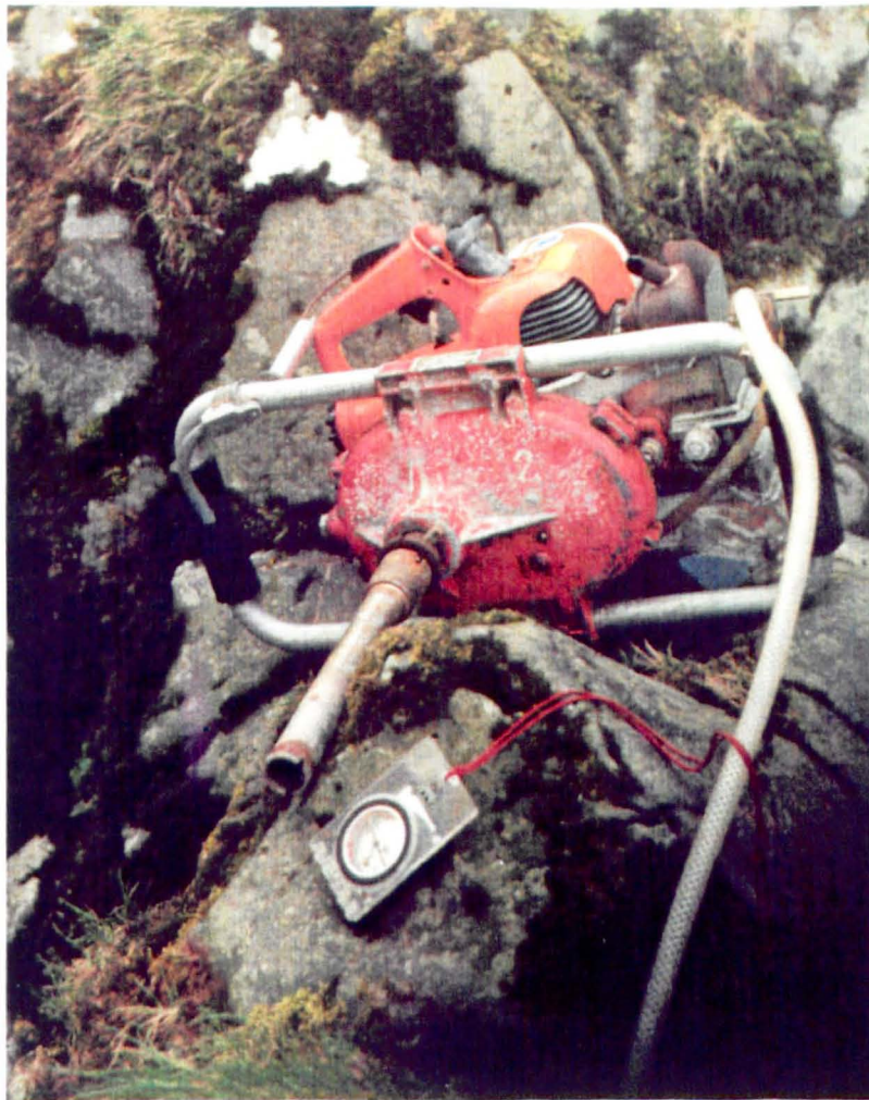
fig.103 Diagram illustrating the orientation convention for palaeomagnetism drilling (in field) and photograph of portable drill in the field.
