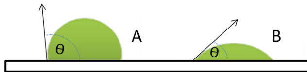
Figure 1.8-2: Surface tension illustration
