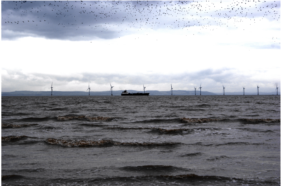
Figure 2.2: A view from the Liverpool Bay Coastal Observatory Formby radar showing multiple clutter sources (March 2010).
