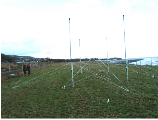
Figure 4.2: HF WERA radar square transmit antenna array, Llanddulas March 2003. Image taken from the NOC archive at http://cobs.pol.ac.uk/wera/photos/ .
