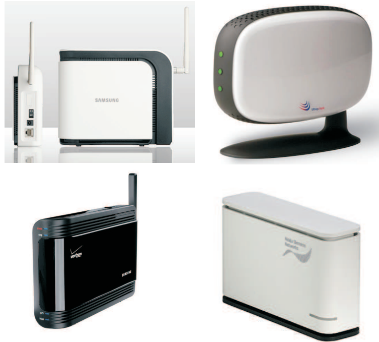
Figure 1.3: Examples of four stand-alone femtocells, manufactured by Samsung, Ubiquity and Nokia Siemens Networks.
