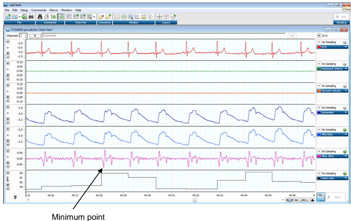
Figure 3.8. LabChart software (LabChart 7.0, ADInstruments) for recording and analysing pulse pressure waveforms for calculation of PWV. The pulse pressure waveforms captured using a tonometer are recorded in channel four. These signals are low-pass filtered at 50 Hz to eliminate noise (channel five) and subsequently band-pass filtered (5-30 Hz) to delineate the foot of the pulse wave (channel six). The minimum point of this signal is the foot of the pulse pressure waveform (depicted by the arrow).
