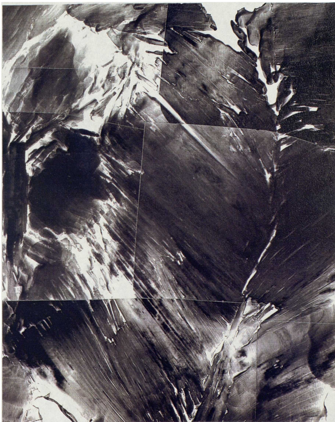
Figure 5.17. TEM montage showing cross-sectional morphology and size of typical kaolinite grains observed in pore space in samples outside of domain 4 (sample 49517A). Identified by qualitative microanalyses. Scale bar 2 \mu\text{m} .
