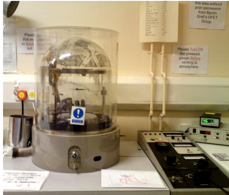
Figure 3.4: Photograph of (a) the metallic thermal evaporator used for the deposition of Permalloy and (b) the organic thermal evaporator used for the deposition of tetracene and other organic materials.
