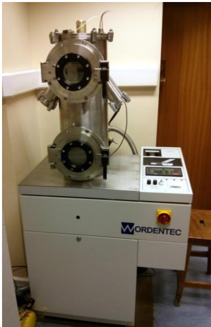
Figure 3.4: Photograph of (a) the metallic thermal evaporator used for the deposition of Permalloy and (b) the organic thermal evaporator used for the deposition of tetracene and other organic materials.
