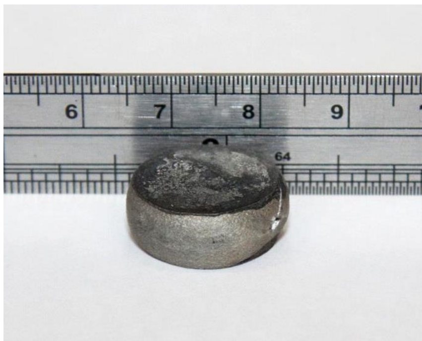
Figure 4.17 – Example of a well deformed sample. Alloy 94 deformed at 450 °C with a strain rate of 1/s.
