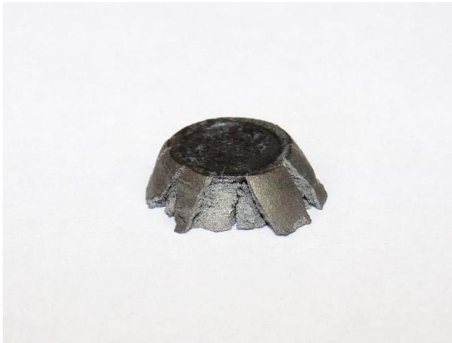
Figure 4.18 – Example of a failure due to shear fracture. Alloy 94 deformed at 425 °C with a strain rate of 5/s.
