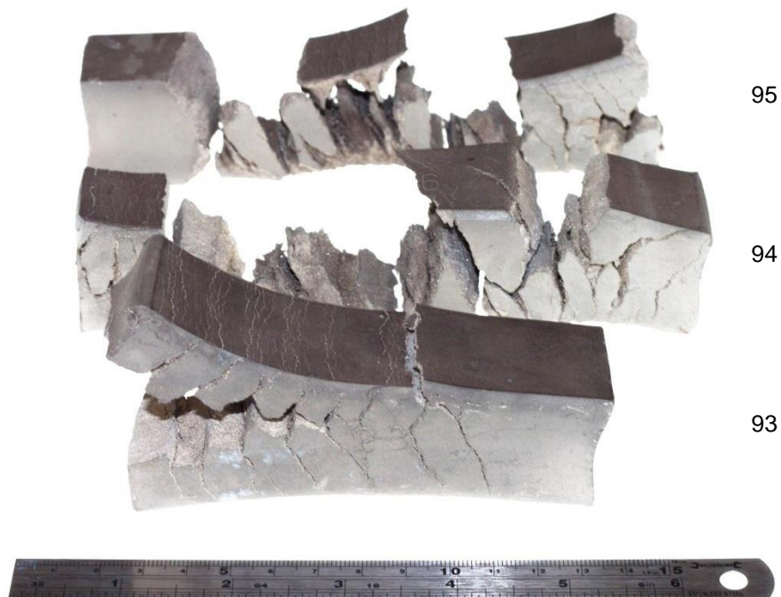
Figure 4.23 – Failure of novel alloys upon rolling at 435 °C.
