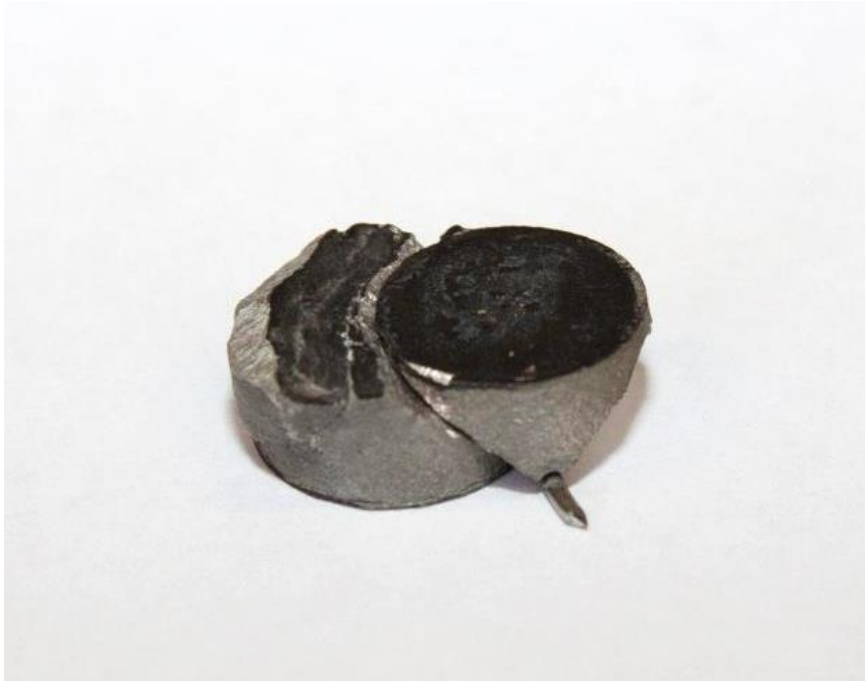
Figure 4.18 – Example of a failure due to shear fracture. Alloy 94 deformed at 425 °C with a strain rate of 5/s.
