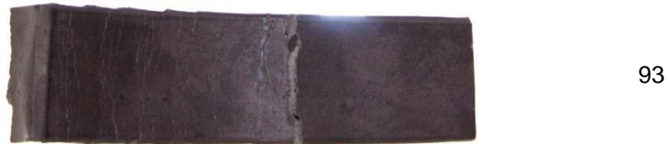
Figure 4.24 – Failure of novel alloys upon rolling at 435 °C (plan view).
