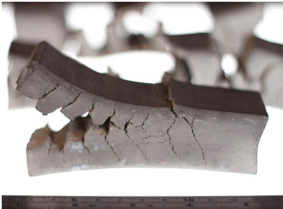
Figure 4.25 – Close up of alloy 93 after rolling at 435 °C.
