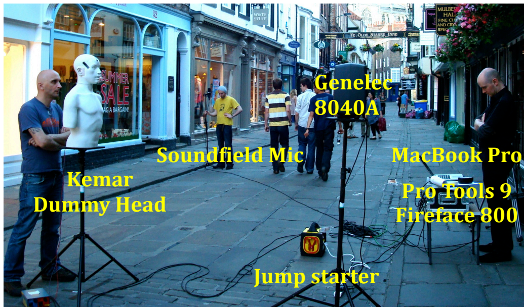
Figure 4.17 – Setup for Acoustic Measurements in Stonegate as part of a pilot study (June 2011).
