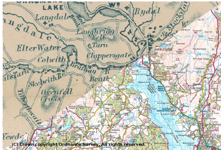
Figure 2.5: Careful creation of visual levels allows the cartographer to overlay several classes of information while avoiding clutter. This figure shows a comparison of map-making technologies from c.1850 with a contemporary design at the same scale. (Copyright Ordnance Survey, used with permission).
