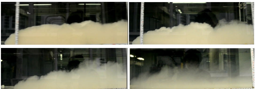
Figure 5.12 Photographs showing the flow of C500 from Series B at t = 5, 12, 23, 58 (top left, top right, bottom left, bottom right, respectively).
