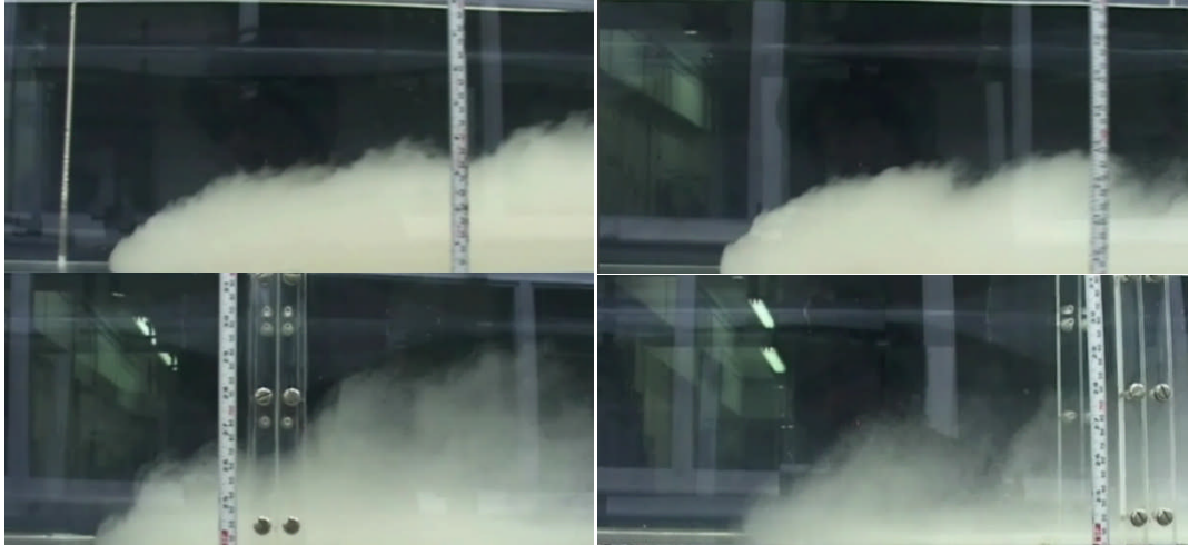
Figure 5.10 Photographs showing the flow of S115 from Series A at t = 5, 10, 15 and 20 s (top left, top right, bottom left, bottom right, respectively).
