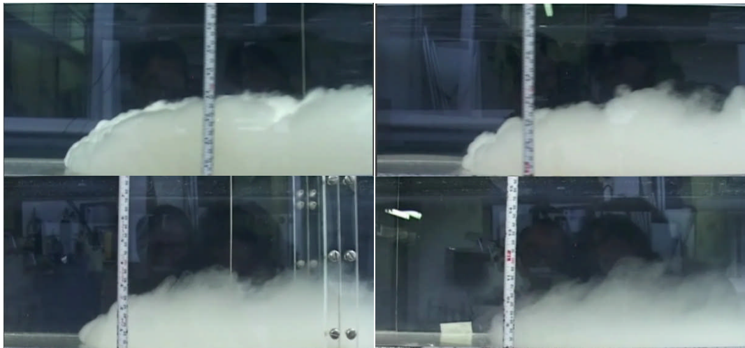
Figure 5.9 Photographs showing the flow of S58 from Series A at t = 10, 20, 30 and 40 s (top left, top right, bottom left, bottom right, respectively).
