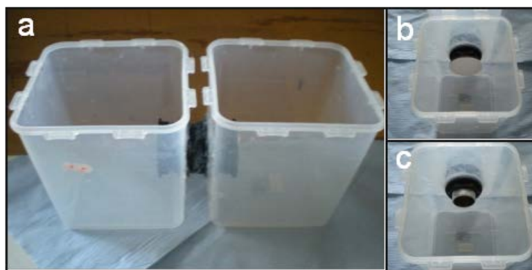
Figure 2.3. Microcosm unit with 0.45 \mu\text{m} mesh fitted to the 'back-nut' (a,b) and with no mesh fitted (c).
