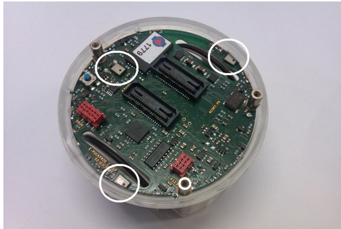
Figure 7.1: The positioning and size of the microphones built into the e-puck
