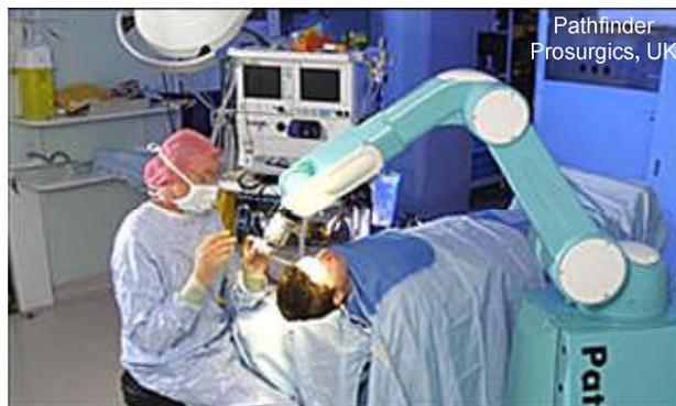
Figure 23. The Pathfinder needle guiding robot for neurosurgery[127].
