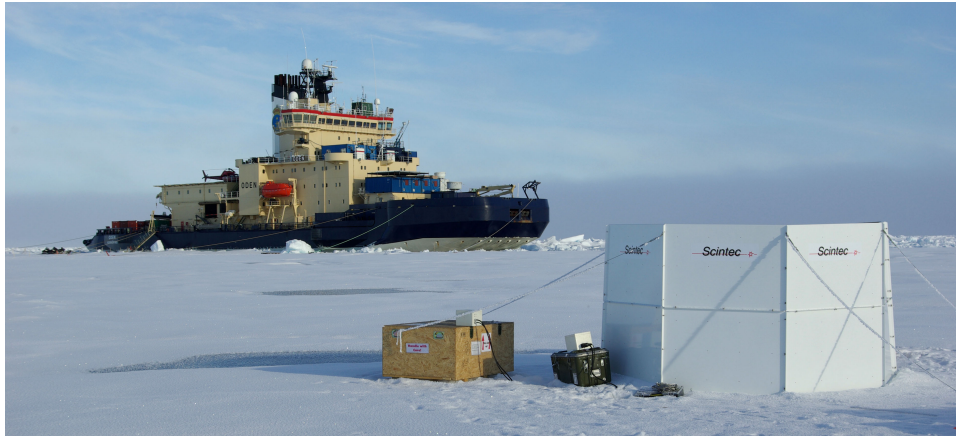
Figure 5.1: The Swedish icebreaker Oden drifting with a central Arctic ice-flow, and in the foreground, acoustic screens around sodar instrumentation. Courtesy of Ian Brooks.
