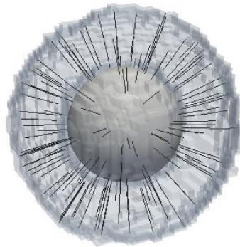
Figure 3.4.10 A nematic shell with homeotropic anchoring at both surfaces showing a defect free director configuration for potential 1, nematic shell thickness of 10\sigma
