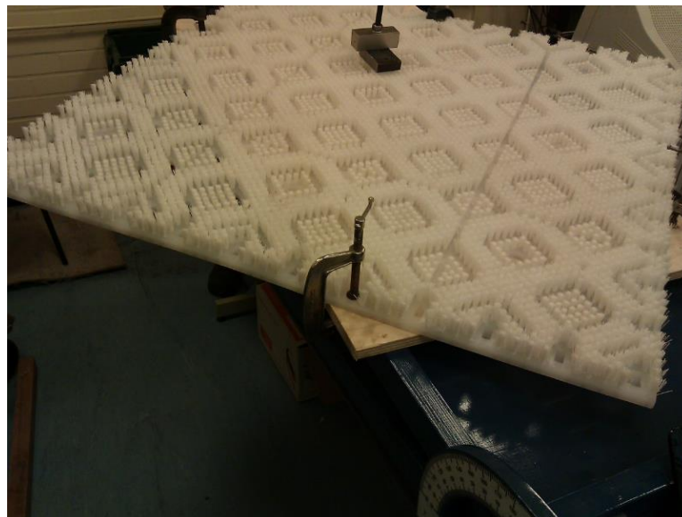
Figure 23: Image of the inclined plane, friction ramp with attached Proslope™ surface and sliding block.
