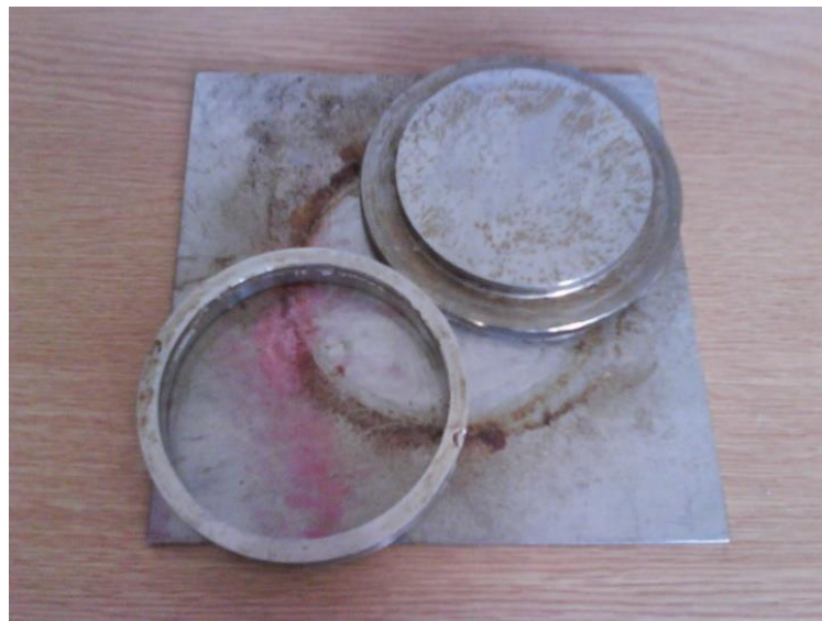
Figure 59: Image of the stainless steel Mould 1 after extended use.
