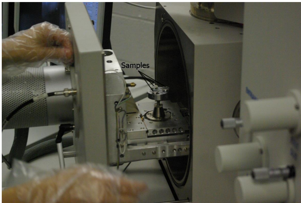
Figure 21: Shows the UHMW-PE samples being placed into the SEM chamber.
