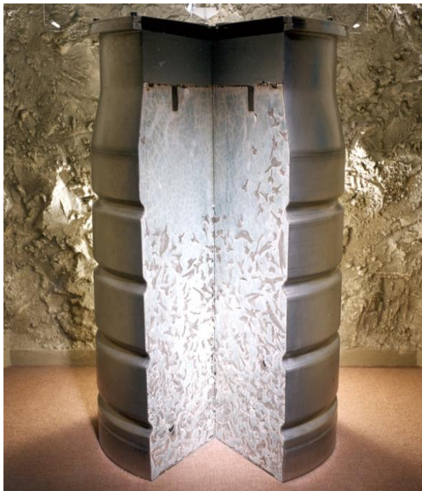
Figure 2.9 Cement-encapsulated solid ILW in 500 L drums. [47]
