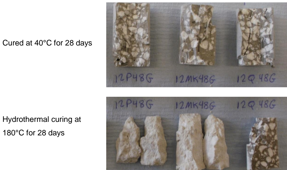
Figure 6.16 PC-mineral admixture samples cured at 40 °C and cured under hydrothermal condition at 180 °C
