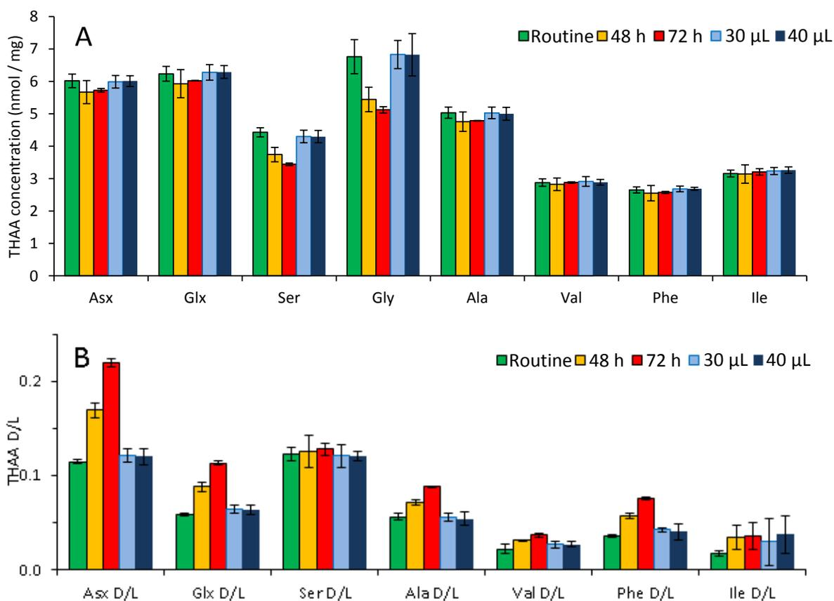
Figure 3.2: THAA concentration (A) and degree of racemization (B) observed for modern OES samples (48 h bleached) prepared using different hydrolysis methods. Error bars indicate 2 x standard deviations based on triplicate samples
