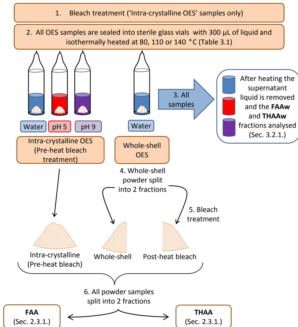
Figure 3.1: Experimental summary for high temperature studies in Chapter 3; FAAw = free amino acid concentration in the supernatant water; THAAw = total hydrolysable amino acid concentration in the supernatant water.
