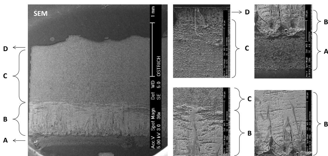
*Figure 2.1: Scanning electron microscopy (SEM) images of a cross-sectional plane of OES: A, organic membrane (removed prior to heating and AAR analysis); B, cone layer; C, palisade layer; D, crystal layer (external surface of the OES). The different calcitic layers were not discriminated in this study. Images kindly supplied by Mary Fairweather and Renée van de Locht of the University of York.*
