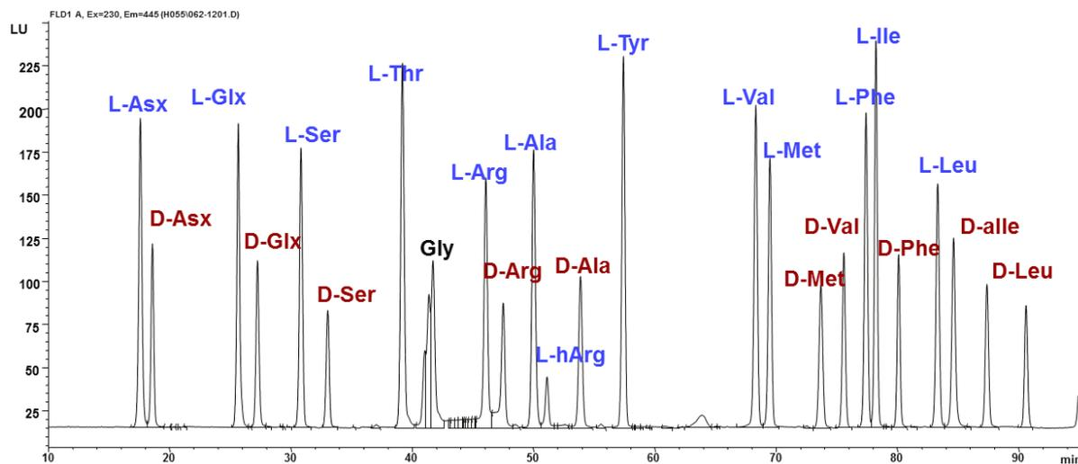
Figure 2.2: Typical HPLC chromatogram of an external standard solution
