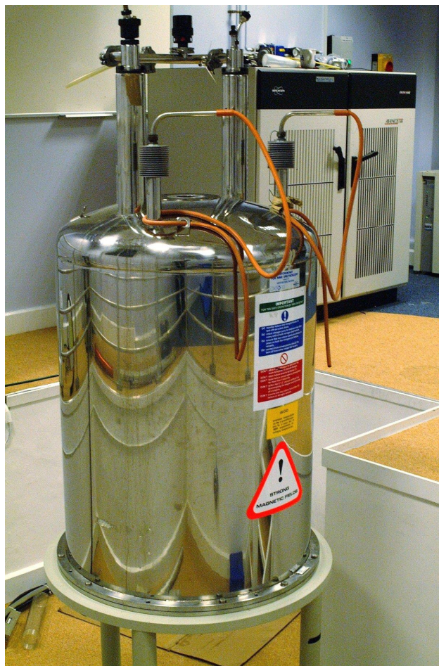
Figure 2.3: Bruker 500 MHz NMR spectrometer , equipped with a TXI 5 mm triple resonance high resolution probe with z gradient.
