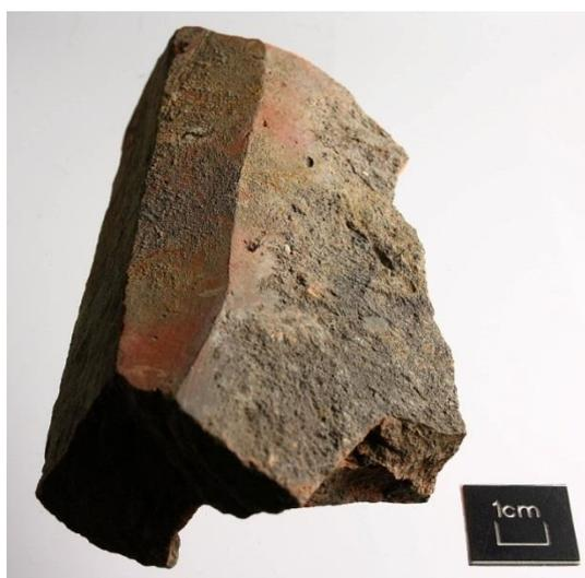
Figure 69. Tegula with either heavy trimming along the arris or an unusual lower cutaway, 1-9 Micklegate Context 6076, ©YAT
