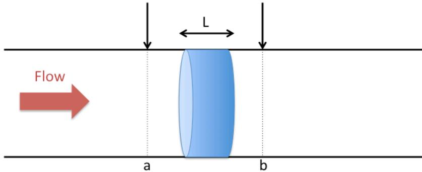
Fig 2.8; A physiological pressure transducer was used to measure the pressure drop before the flow enters the scaffold (point a) and immediately after it leaves (point b) for flow rates of 3, 5 and 10 ml/min.
