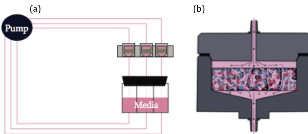
Fig 1.13; (a) Schematic of the 8-chamber flow-perfusion bioreactor within a standard cell culture incubator. (b) Schematic chamber within the flow-perfusion bioreactor whereby media is forced through the entire structure of the scaffold. Arrows indicate direction of flow [216].
