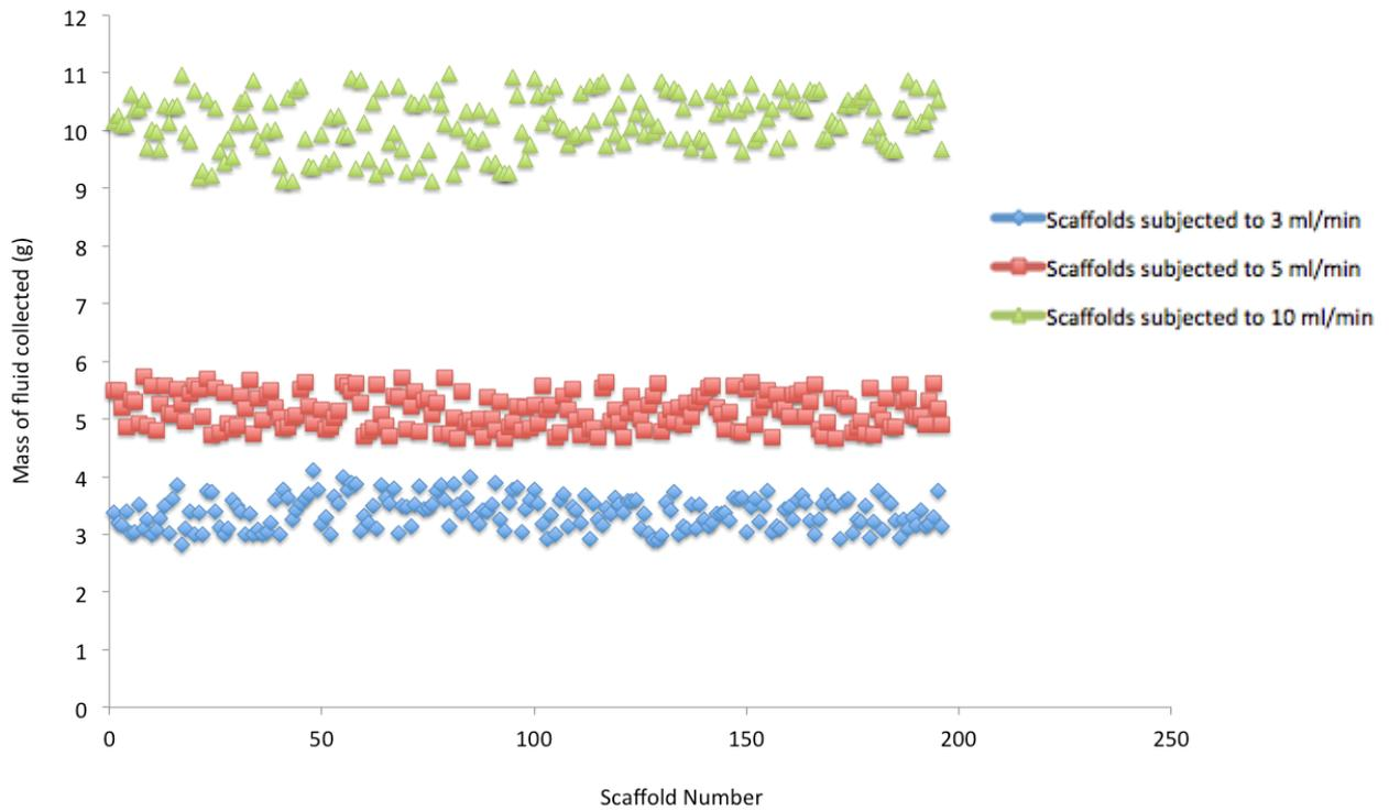
Fig 2.6; Scaffold geometry was roughly estimated using a time-collection method with the peristaltic pump. Individual scaffolds were subjected to flow rates of 3, 5 and 10 ml/min for one minute. The fluid would then be collected in a small tub and weighed. The blue, red and green dots represent the amount of fluid collected for scaffolds subjected to 3, 5 and 10 ml/min respectively.
