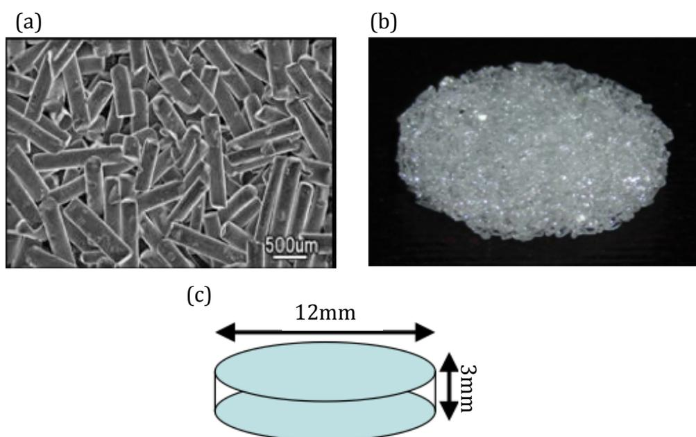
Fig 2.2; (a) Image of cylindrical glass rods, which are sintered to create randomly oriented glass scaffolds. The result is a highly porous material, with pores of variable size making up approximately 60% of the total volume. (b) image of a single glass scaffold (c) dimensions of a single glass scaffold (12 mm x 3 mm).
