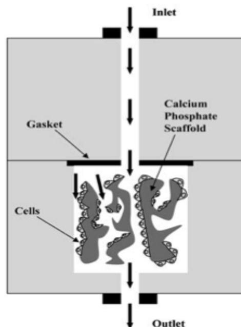
Fig 1.15; Schematic drawing of the chamber within the flow-perfusion bioreactor. Media is forced through the calcium phosphate scaffold providing fresh media and subjecting cells to a mechanical stimuli. Arrows indicate direction of flow [84]
