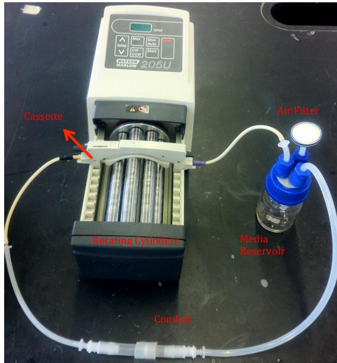
Figure 2.4; Photograph of the peristaltic pump system. Rotating cylinders pump media from the media reservoir towards the conduit in which scaffolds were held in place.
