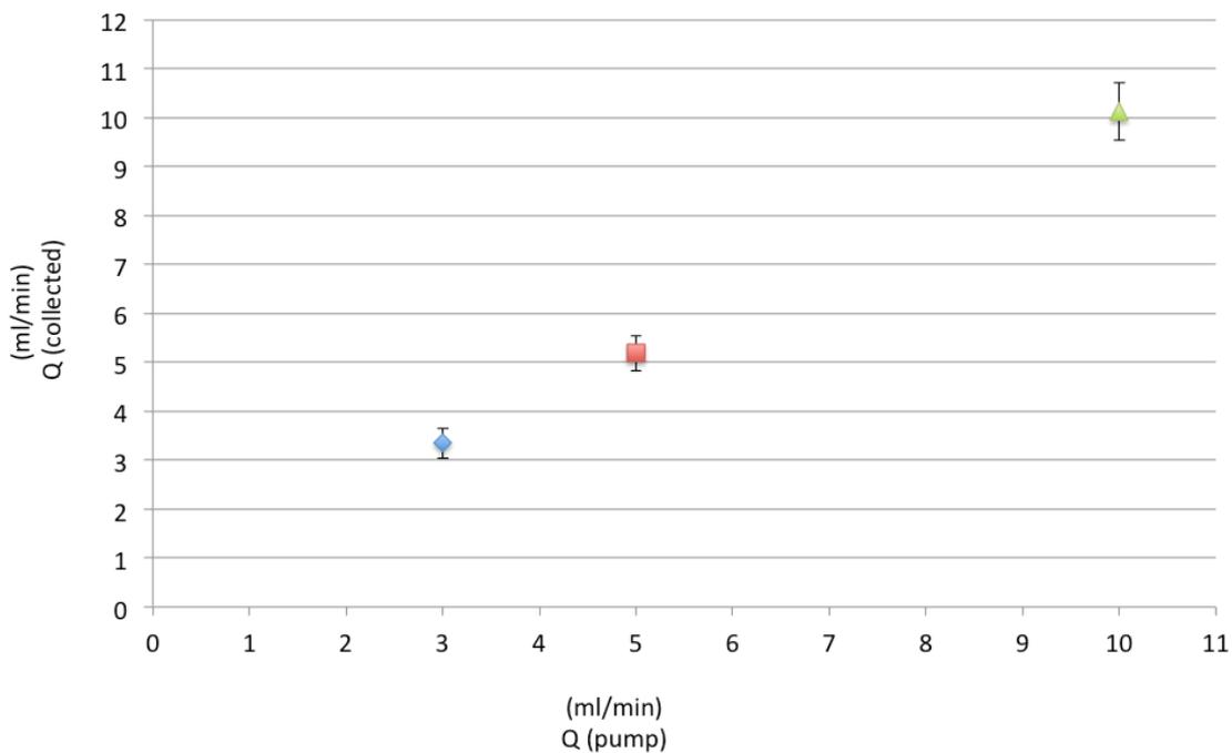
Fig 2.7; Results from the time-collection method were used to compare the actual flow rate ( $Q$  collected) to the flow rate applied by the pump system ( $Q$  pump). Scaffolds subjected to 3 (blue), 5 (red) and 10 ml/min (green) produced a flow rate of  $3.352 \pm 0.309$ ,  $5.19 \pm 0.361$  and  $10.12 \pm 0.584$  ml/min respectively.
