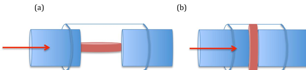
Fig 4.1; Scaffolds where subjected to fluid flow whilst positioned in two different planes. (a) Horizontal plane (parallel flow, whereby the direction of flow is parallel to scaffold surface), (b) vertical plane (transverse flow, whereby direction of flow is perpendicular to scaffold surface). Arrows indicate direction of flow.
