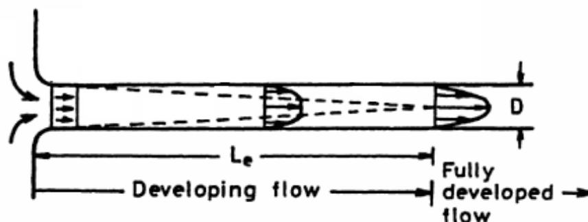
Fig 2.5; Flow in the entry region for laminar flow.
