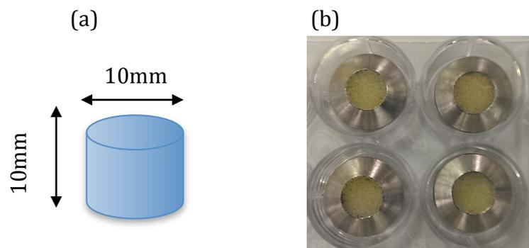
Fig 2.1; (a) The dimensions of a single PU scaffold and (b) PU scaffolds were hole-punched, sterilized and washed with PBS. Steel rings held the PU scaffolds in place for the for initial cell seeding which contained 100 µl media with 500,000 cells per scaffold.
