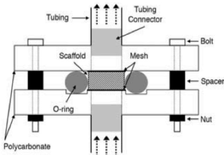
Fig 1.14; Cross section of the scaffold chamber. O-rings hold cell-seeded scaffold in place whilst media is pumped through the tubing. Arrows indicate direction of flow [85].
