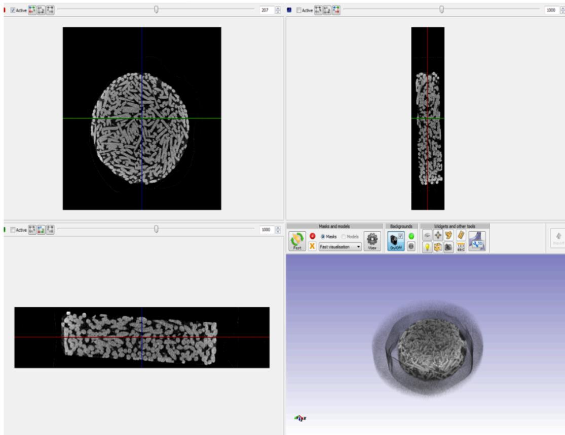
Fig 7.1; Micro-CT images of the glass scaffold was obtained by placing the scaffold in a SKYSCAN 1172 micro-CT machine. This resulted in a total of 415 images taken from top to bottom of glass scaffold. Images were compiled in ScanIP to create a 3D model.
