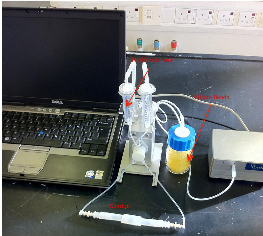
Figure 2.3; Photograph of the IBIDI oscillatory pump system. All tubing were sterilized in advance to prevent contamination. A single scaffold would be placed in the conduit and subjected to fluid flow for 1 hour at a frequency of 1 Hz.
