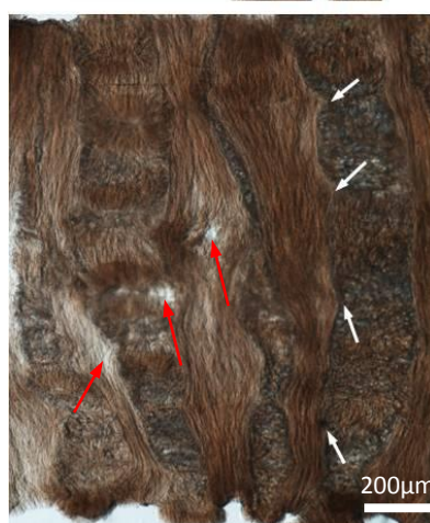
Figure 7.12 - Micrographs from tensile test sample T2 showing the specimen prior to loading (top) and the specimen loaded (bottom) with an extension of 4mm. The white arrows show an example of a lamellar boundary that has become puckered at the locations at which it intersects the interlamellar bridging elements. The red arrows indicate areas of lamellae that have thinned.
