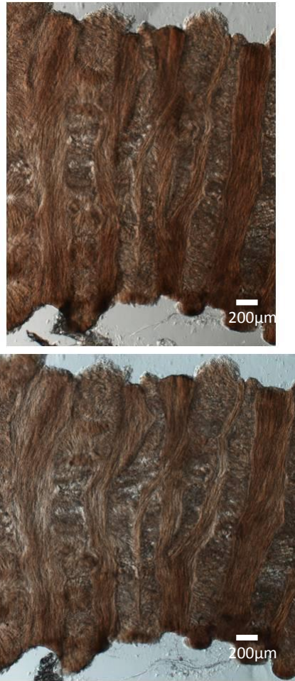
Figure 7.11 - Micrographs from tensile test sample T1 showing the unloaded specimen (top) and the specimen loaded (bottom) with an extension of 3mm.
