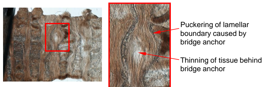
Figure 7.28 – Detail of test T3 in the loaded state. The lamellar tissue is seen thinning and fibres are pulled apart within the lamella's fibre bundle adjacent to the anchor point of the minor bridge. This is the initiation of cleft formation.
