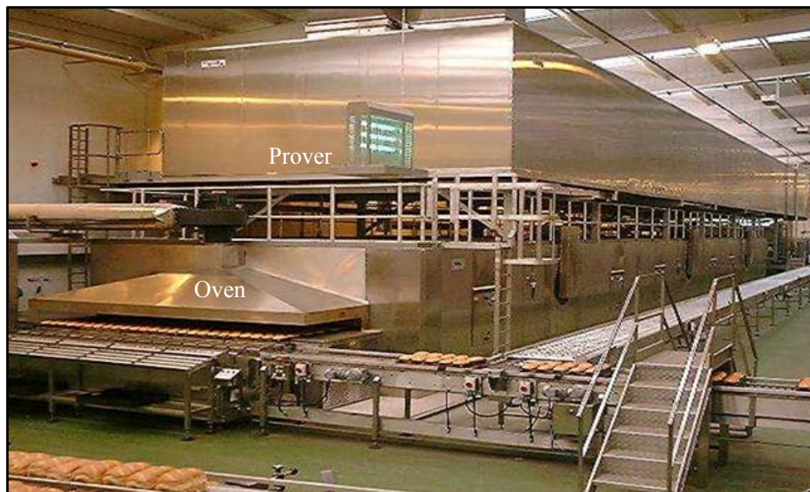
Figure 1.4 – Photograph of an industrial bread prover located above an industrial oven (Warburtons Limited and Spooner Industries Ltd.)
