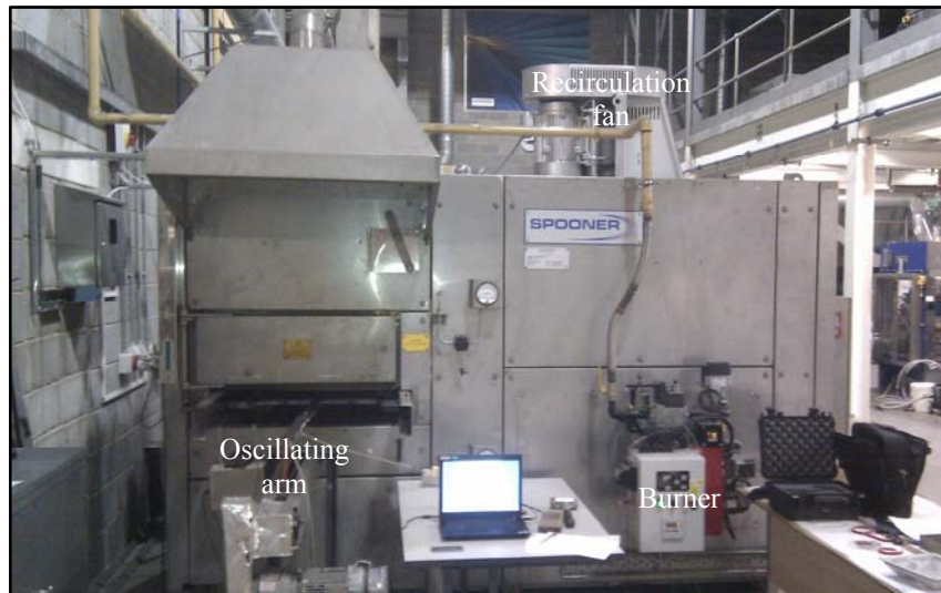
Figure 7.1 – Partially labelled photograph of the pilot oven used for heat transfer experiments
