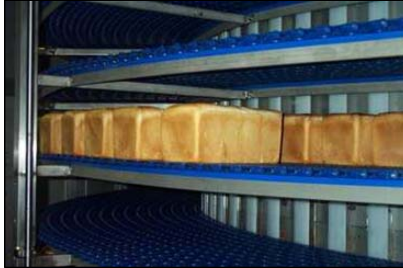
Figure 1.6 – Photograph of the inside of a spiral bread cooler (Spooner Industries Ltd.)
