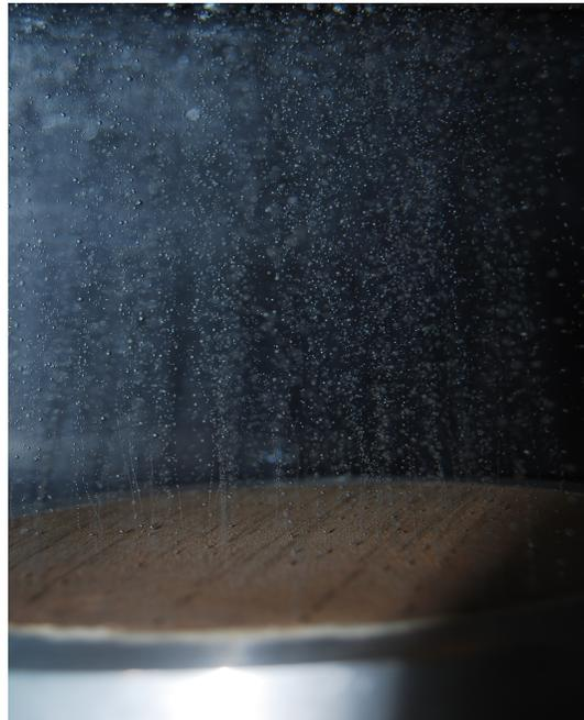
**Figure 4.1:** Photograph of microbubble generation from a ceramic diffuser with 20 µm pore size. Average bubble size produced was ~300 µm, 15 times larger than the diffuser pore size.
