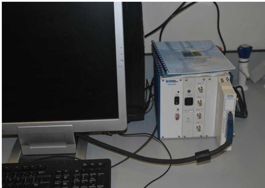
**Figure 1:** Photograph of the multi-system acoustic bubble sizer. The set consists of an interface where hydrophones (Transmitting and Receiving) are connected. Signals at set frequencies are sent via the transmitting hydrophones with the receiving hydrophone positioned directly opposite the transmitting hydrophone but across the rising bubble cloud, to collect the attenuating signals from where bubble size can be estimated.
