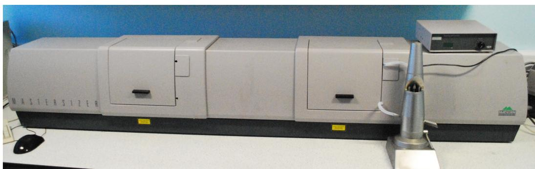
**Figure 2:** Picture of the Mastersizer used for particle size measurements. Incident laser beam is scattered as it passes through a dispersed sample containing particles. Small particles scatter light at higher angles while larger particles at smaller angles relative to the incident laser beam. The instrument collects the scattered light at different angles and based on the Mie theory of light scattering, an estimation of the particle size is made.
