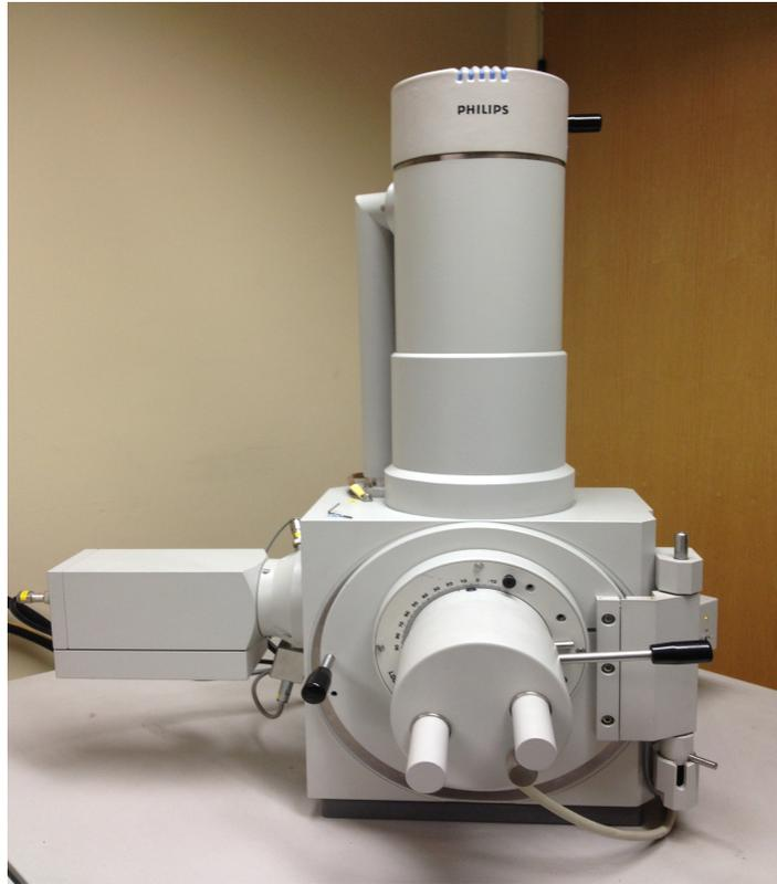
**Figure 5:** Photograph of the Scanning Electron Micrograph (SEM).
