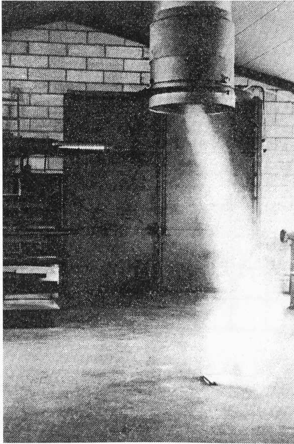
Fig.1.5 The Aaberg ventilator unit suspended 3.5d above the floor. Smoke is released on the floor beneath the ventilator.
