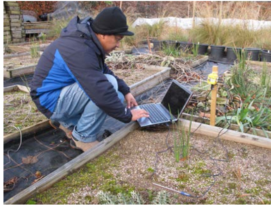
Figure 4.3 Data downloaded every month from TinyTag data logger in experimental plot.
