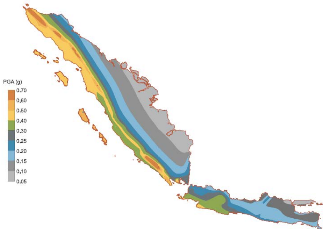
Figure 2.9. Seismic hazard map of Sumatra at 10% probability of exceedance in 50 years on rock site (Irsyam et al., 2008)
